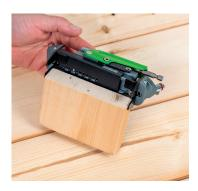
1. Adjust the tool according to the width of the board by pulling the grey button on the top of the tool.
